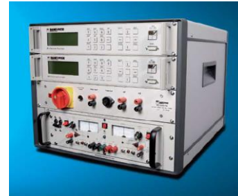
REMACOMP ® -REMACOMP ® combination C - 710 with two electronic fluxmeters EF 5. (The stand-alone computer is not shown.)
