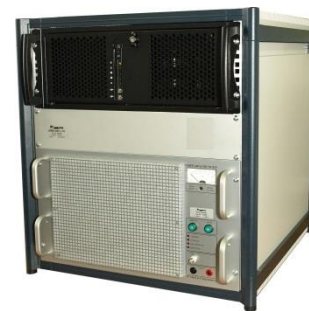
Cabinet of REMACOMP ® C - 100, housing power amplifier and computer
